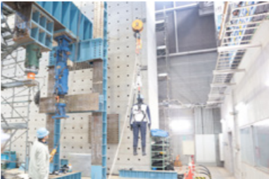
Risk simulation training (Experimental crash test of a dummy using a fall-control device)
