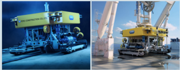
Subsea cable ROV trencher (Photo provided by SMD)
