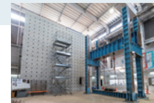
Reaction wall (left) and Large scale loading frame (right)
