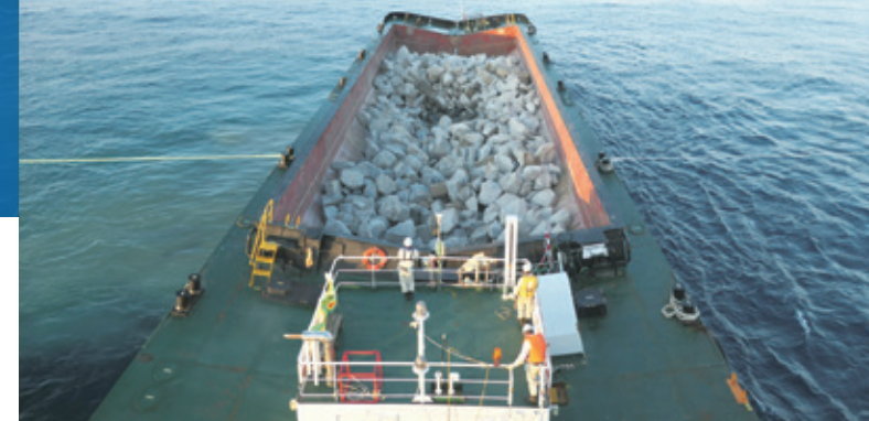
Dedicated vessel to throw in stone material to the seabed. The ship's bottom (shown at the top of picture) will open, and stone material will be thrown in.
