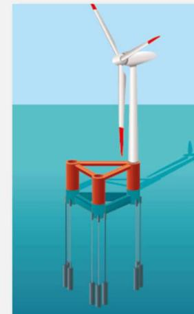
※ Attached by tension of wires from seabed
