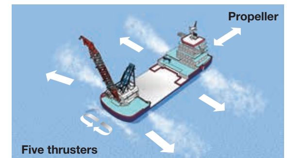
Conceptual illustration of the DPS (Dynamic Positioning System) motion
