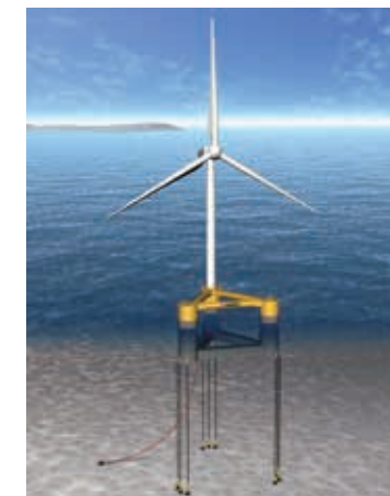
Conceptual drawing of TLP method (Source: MODEC, Inc.)
