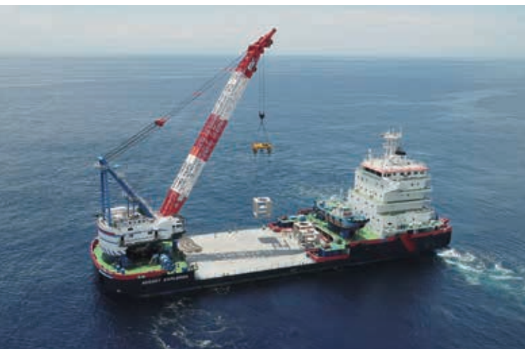
AUGUST EXPLORER, having capability of navigation without stopping at a port for a long time, and equipped with a state-of-the-art fixed-point retention function that enables works in strong winds or strong underwater currents.
