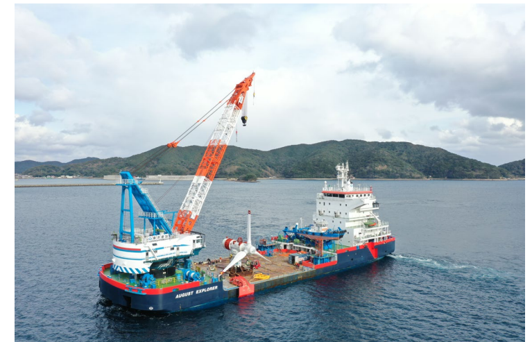
The Underwater installation of Japan's first commercial-scale large tidal turbine (on the ship) in the Goto Islands Nagasaki prefecture, in utilizing our self-propelled multipurpose vessel 'August Explorer'
