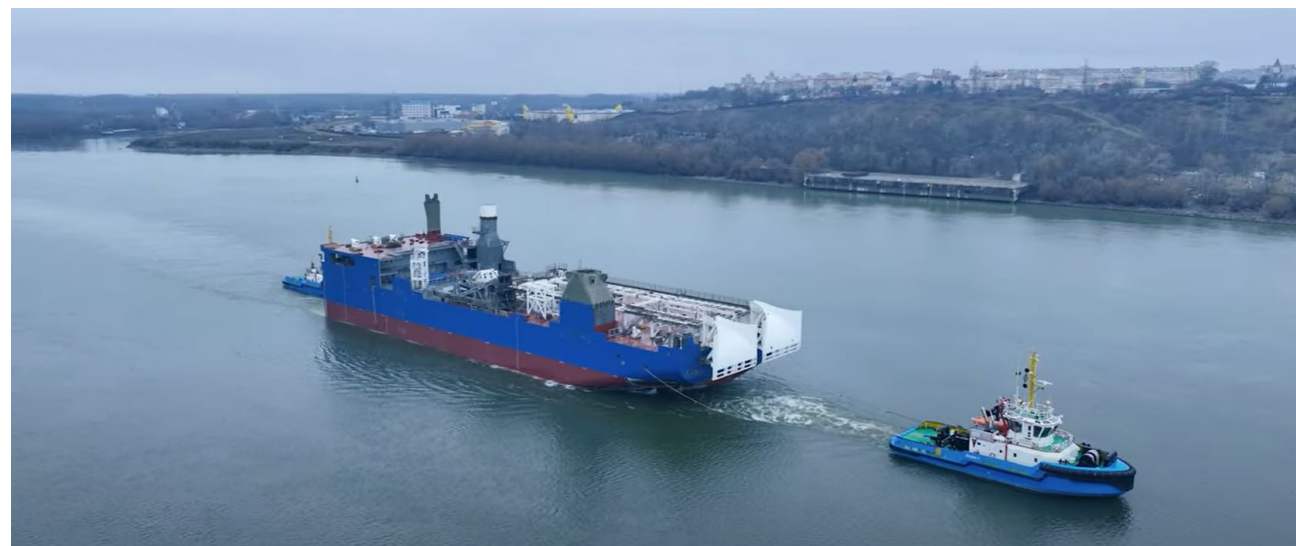
CLV under construction
