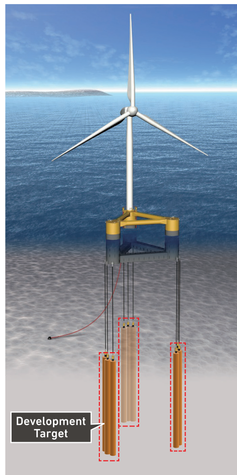
Schematic diagram of TLP method (Courtesy of MODEC, Inc.)
